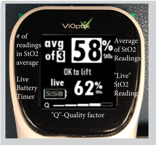
**Time**- Need to leave the device on tissue at least 5 seconds to stabilize reading
